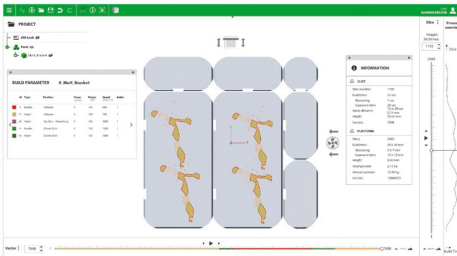
**6 Viewer.** The last step before production is the examination of the slices that have been created. The various slice areas of Volume, Border, Down-Skin and Up-Skin are visualized for better depiction in various colors. After the verification, the processed data are exported into a desired
