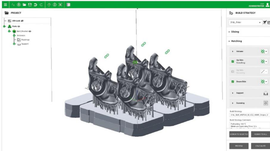
**4 Nesting.** Multiple instances (copies) of a part are reproduced as a matrix model. Changes are transferred via a mother-child relationship 1:1 to the instances which guarantee identical construction parameters.
